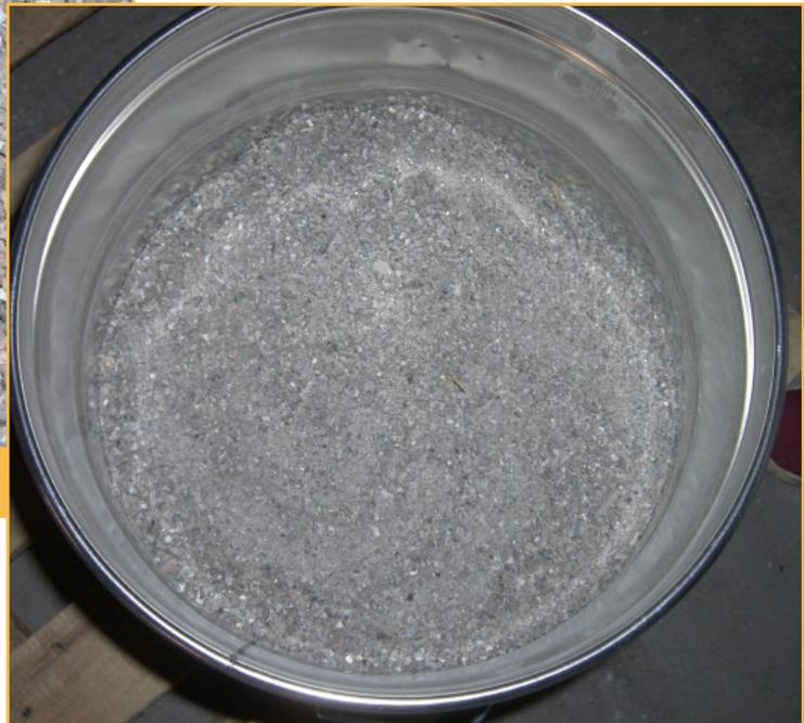
Among its many metallurgical uses, calcium carbide has been found by EAF shops to be an essential tool for the removal of unwanted iron oxide from furnace slag that is carried into the ladle during tapping. Left untreated, these oxides can interfere with the downstream steel refining operation by inhibiting desulfurization, oxidizing (“fading”) alloy additions, and attacking refractories.
